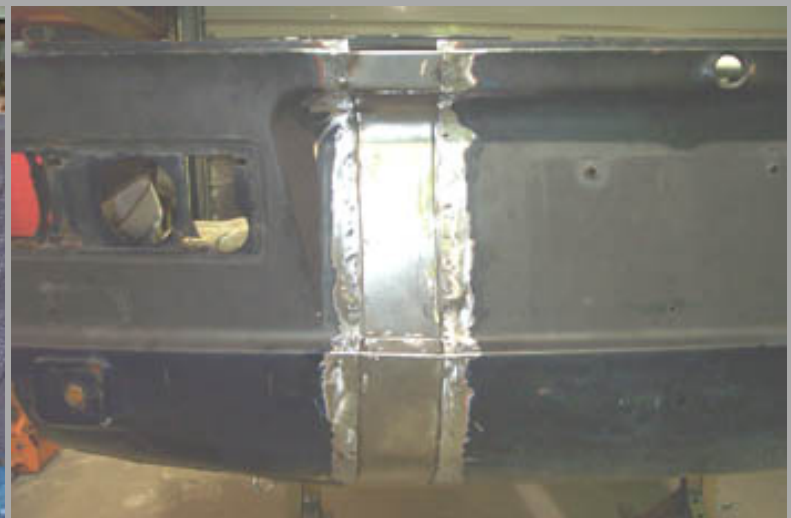
Two 3" pieces of new sheetmetal have been cut, fitted and welded in place on the rear valance thus increasing its overall width by 6" as it should
