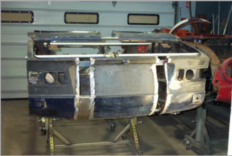
Back valance has been cut in 2 places so as to retain the integrity of the trunk lock mechanism
