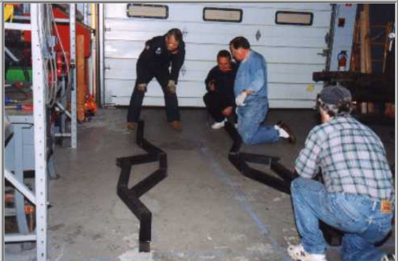
Viola! The angles being calculated and cut correctly make the pieces fit nicely together and duplicate the curves of the old frame
