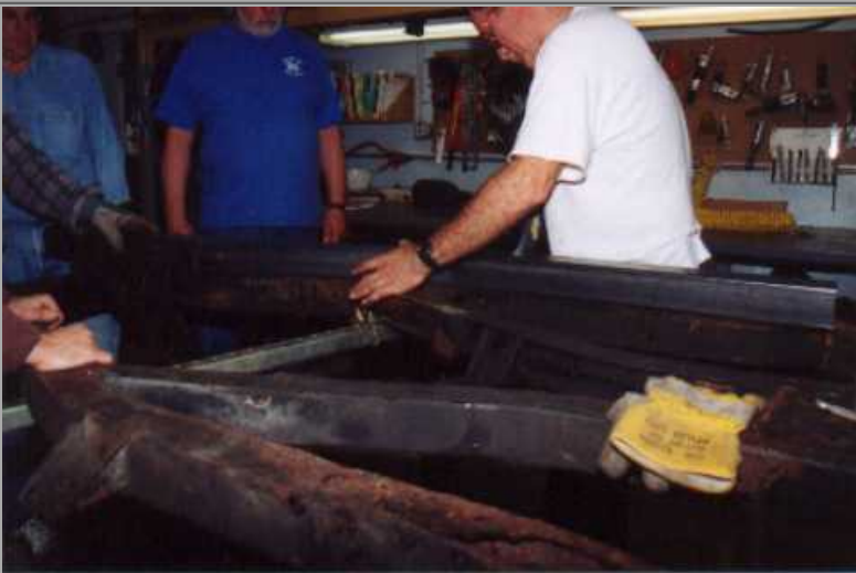
All the frames curvatures would be accomplished by calculating the correct angles to cut the ends of the tube steel then butt and weld the ends together
