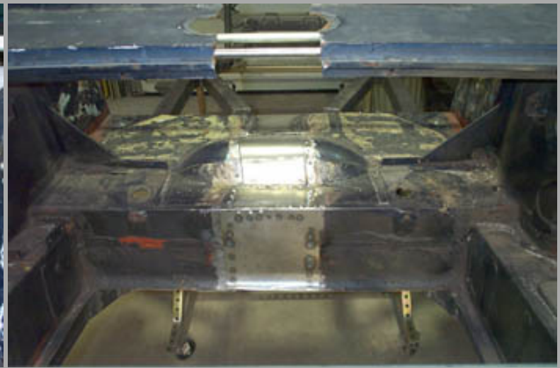
New sheetmetal welded in place at heelboard and rear floor. Since sheet metal has been removed, temporary cross support braces have been installed to keep the integrity of the body straight and intact
