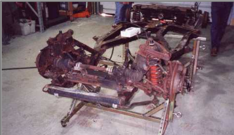
Frame now exposed was studied. Suspension & drivetrain components were removed
