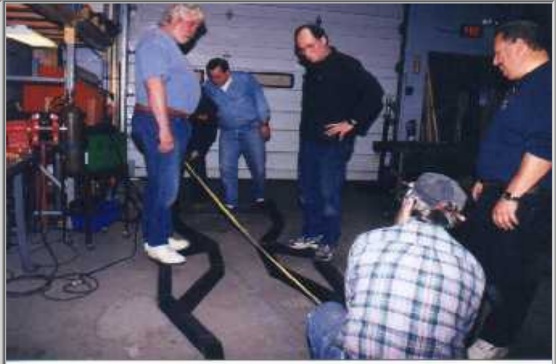
Measurements were taken several times over for frame squareness before the pieces were all spot welded together
