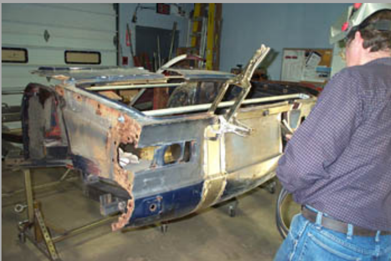
Two 3" pieces of new sheetmetal have been cut, fitted and welded in place on the rear valance thus increasing its overall width by 6" as it should
