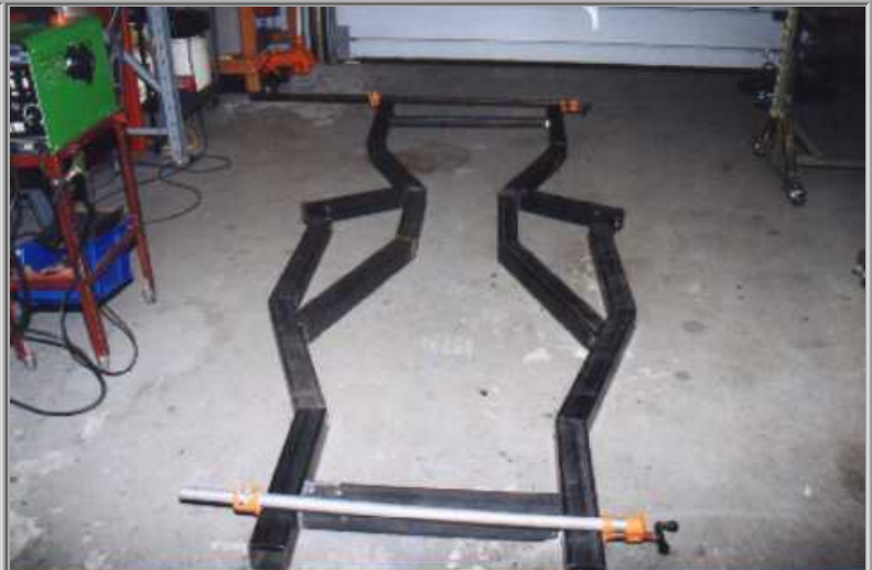
The major portion of the new frame completed with some of the new pieces spot welded in place
