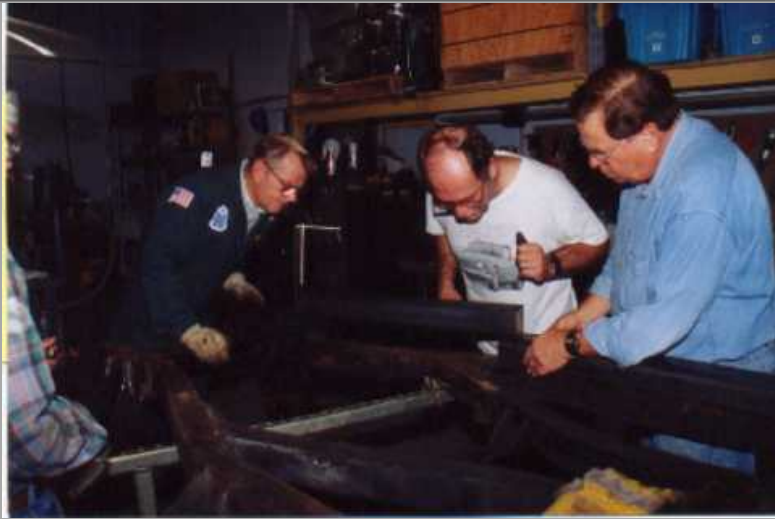
All the frames curvatures would be accomplished by calculating the correct angles to cut the ends of the tube steel then butt and weld the ends together
