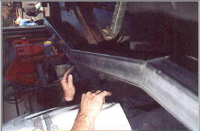
Viola! The angles being calculated and cut correctly make the pieces fit nicely together and duplicate the curves of the old frame
