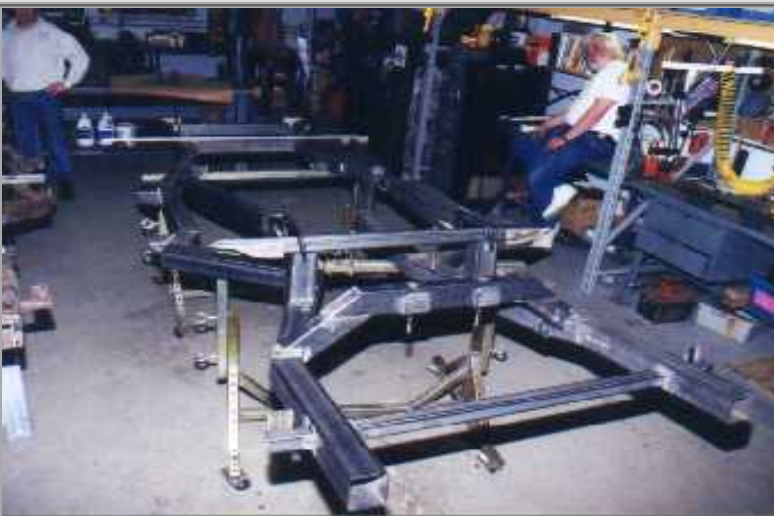
Frame has been squared up to everyone's satisfaction and is awaiting final tack welds
