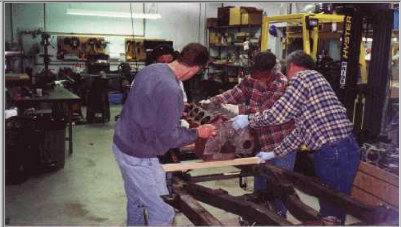
Wood blocks were fastened to the frame and engine was set in place. Engine would fit TR6 as is. When the car is widened, there will be even more room
