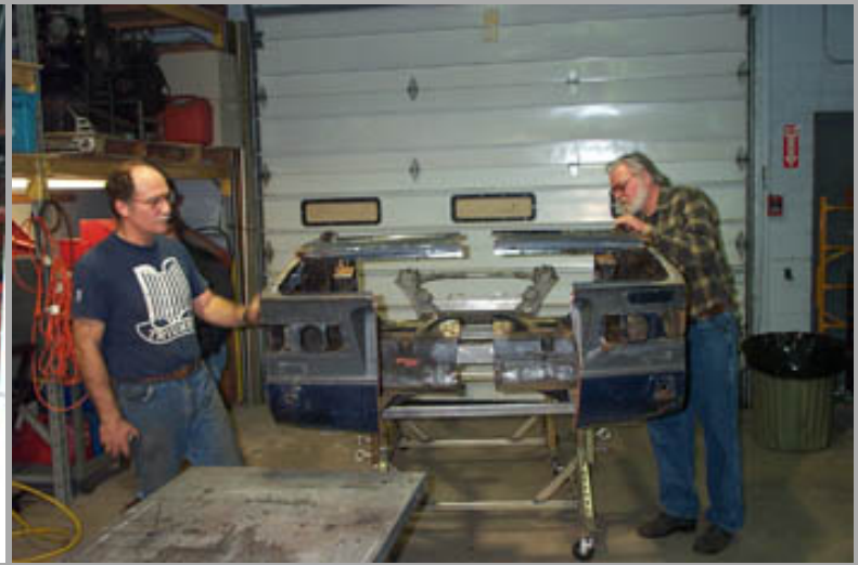
Back valance has been cut in 2 places so as to retain the integrity of the trunk lock mechanism
